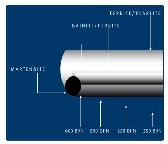
As the distance from the inner pipe wall increases, the hardness tapers and the ductility increases to the outer surface into the pipe wall. As the distance from the inner pipe wall increases, the hardness tapers and the ductility increases to the outer surface.
